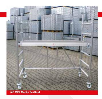
The high-grade aluminium makes the whole mobile scaffold group light and exceptionally durable. The casters with the diameter of 200 mm and 125 mm ensure comfort maneouvering. When the scaffold is put in the desired location you can secure it with the foot brake. Addiotnally, the adjustable jacks ensure precise structure setting by exact structure levelelling. The scaffold is stable due to universal and exapandable mobile beams as well as supports.
